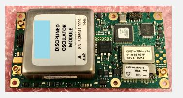
GPS Disciplined oscillator providing 10MHz and 1PPS
