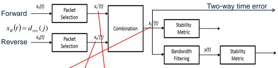
Two-way time error sequence is calculated using the packet-selected time error sequences:
