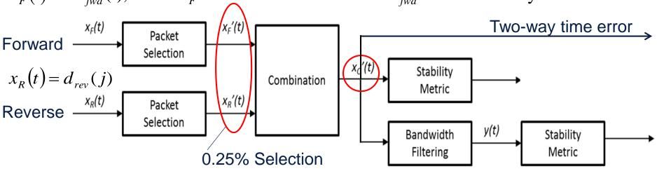
Two-way offset, or two-way time error is calculated using packet selected time error sequences:
