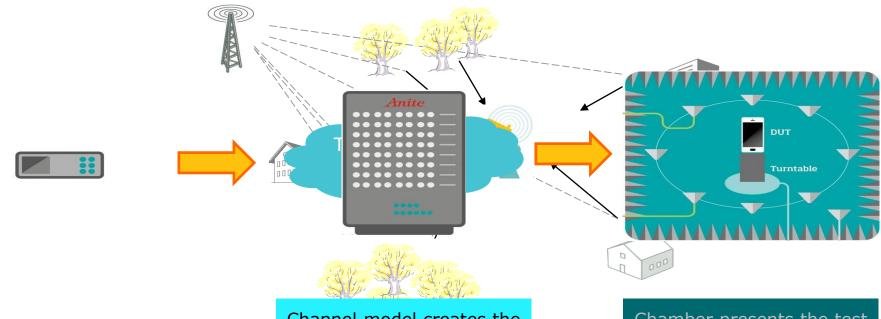
Channel model creates the typical radio conditions in which the DUT operates
