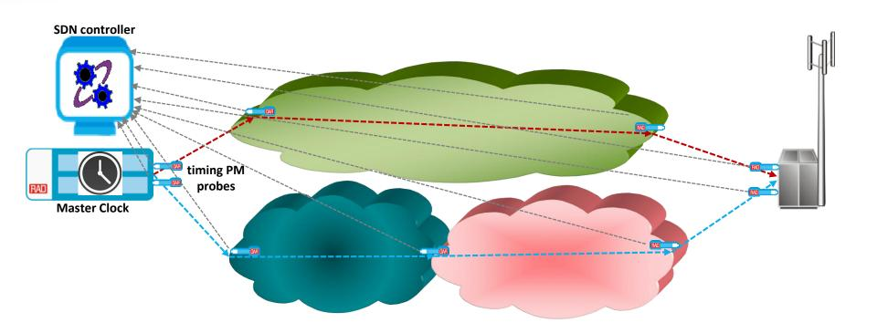
Timing performance probes report to a timing PM portal which computes the timing accuracies expected from each end-to-end path
