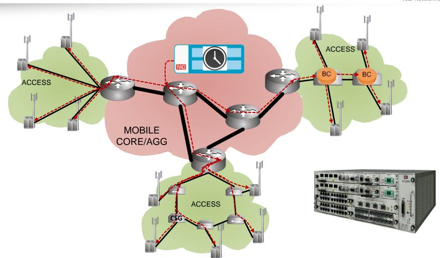
Conventionally there is one centrally located GM per network One must ensure distribution does not overly degrade timing performance On path support (BCs and/or TCs) used as needed
