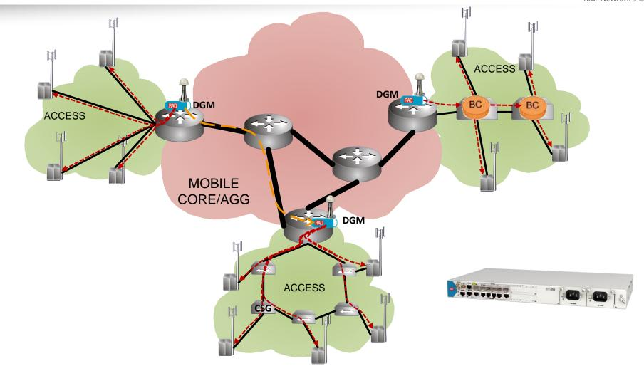
Distribution is less critical if we use Distributed GMs closer to base stations Failures cause less damage, and it is not difficult to share for backup
