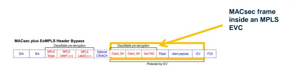
Protects MEF EVC payload while allowing network to push/pop VLAN tags and MPLS labels, as well as mark the frames for SLA-compliance (policing result)
