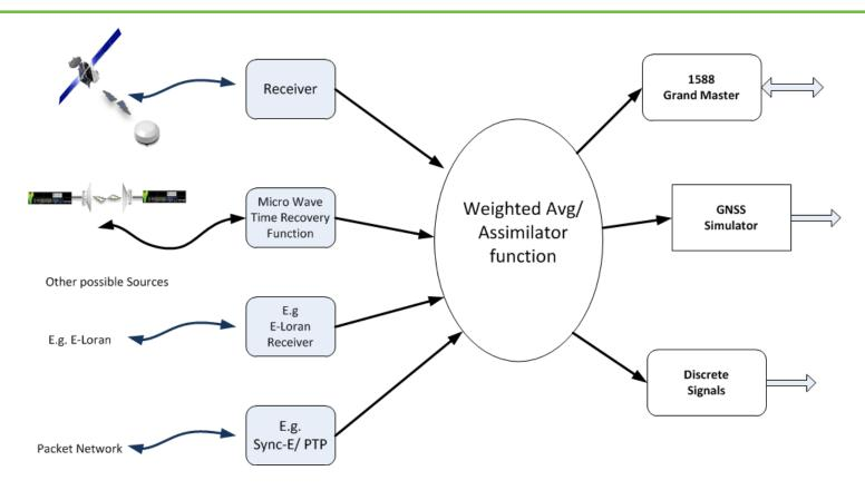
Weighted Averaging of inputs- to generate stable outputs
