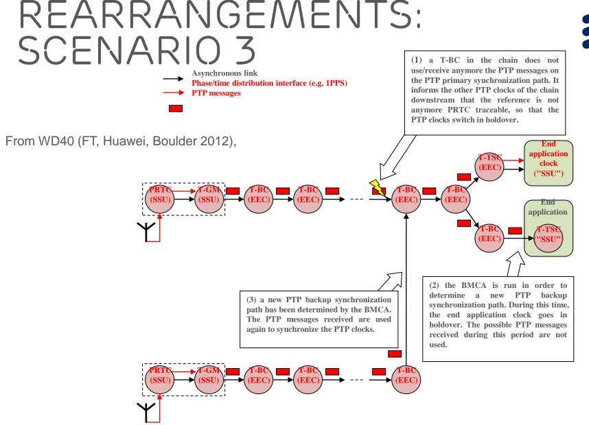
Rearrangements could be controlled within 150 ns assuming the Time clock allows for fast start up If this is not possible a higher budget would be required instead (about 400 ns).
