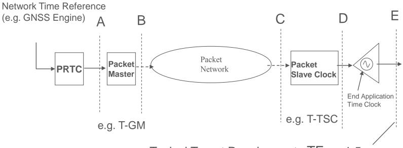
Typical Target Requirements  $TE_E < 1.5 \mu s$  (LTE TDD, TD-SCDMA)
