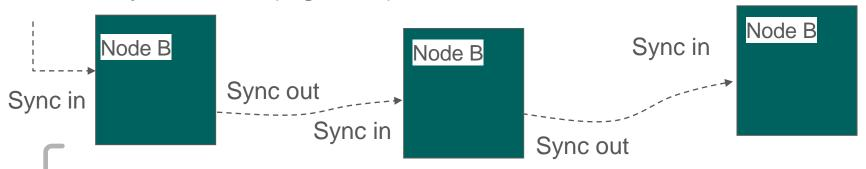
The Requirements is +/-1.25  $\mu s$  for independent inputs to the NodeBs
