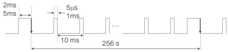
The relative phase difference of the synchronization Signal shall not exceed 2.5  $\mu s$  (3  $\mu s$  is mentioned for TD-SCDMA) External sync Source (e.g. GPS)
