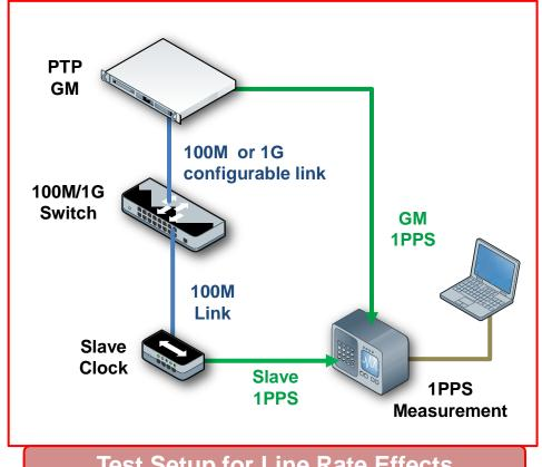
**Test Setup for Line Rate Effects**
