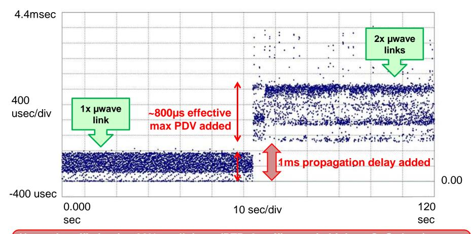
Network traffic load at 90% at all times (PTPv2 traffic was in highest QoS class) 1ms change in propagation delay as effect of added link (symmetric) Large increase in PDV compared to fixed line 'hops'
