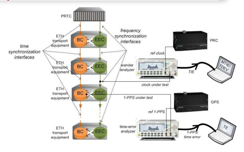
Hop-by-hop → Measurable signal (phase or time error) is easily mapped to meaningful performance metrics (MTIE/TDEV or TE)
