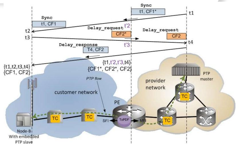
In addition to the timestamps information {t1,t2\*,t3\*,t4}, the ToPDF has all the required correction field information: {CF1\*, CF2-CF2\*}
