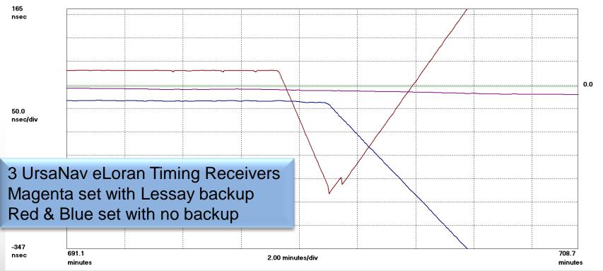
Also proves eLoran in inherently selfresilient to Tx failure.
