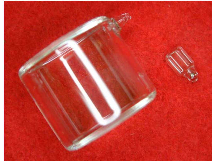
Comparison between classic 1" long (LPRO) and latest ultra-miniature (X72) integrated Rb gas cells
