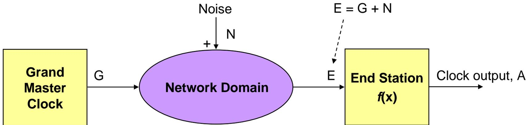
Clock output must meet application requirement,  $A$
