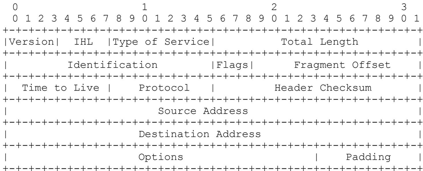
Note that the IPv4 packet is preceded by the datalink header, for example an Ethernet header
