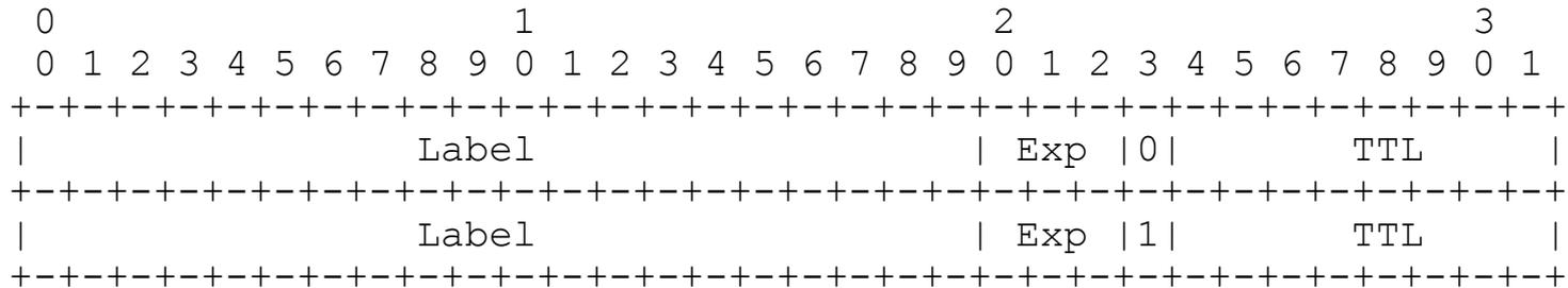
LSE is preceded by a datalink header (e.g. Ethernet) and followed by either an IP header, or a pseudowire payload
