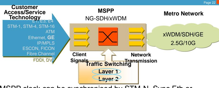
MSPP clock can be synchronised by STM-N, Sync Eth or external synchronisation ports
